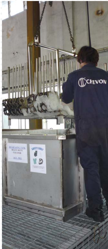
Chemical Cleaning of plates in our Chemical Tanks
