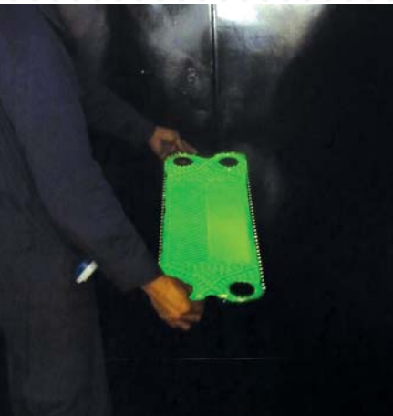
100% Dye Penetrant Test and UV Checking for detection of cracks and pinholes
