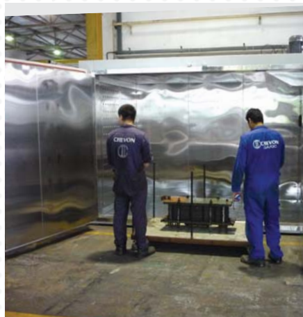
Securing Gaskets onto plates by Oven Curing
