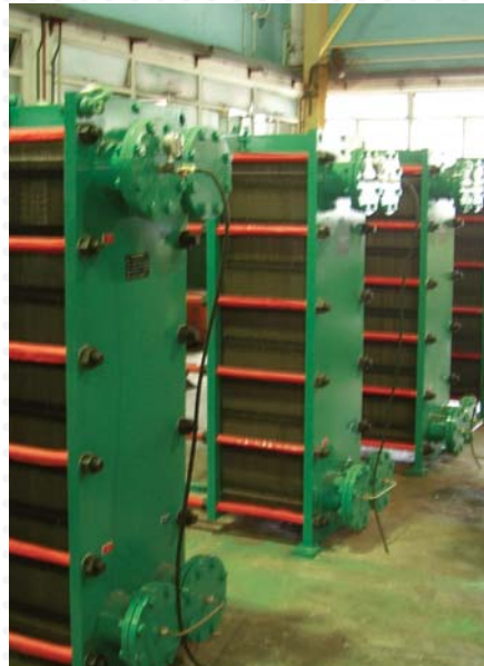
Hydrostatic Testing of Reconditioned/Serviced Plate Heat Exchanger Units
