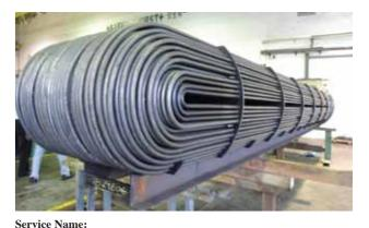
U tube Bundle 957mm OD X 6,038mm L X 388 'U' tubes MOC: SA516-70N End user: Kaduna Refinery Petrochemical Co
