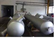
Service Name: Condenser Thermal Oil Cooler Size: 815mm ID x 5,000mm LG x 381 U-tubes of 2.11mm Thk MOC: SA516-70N End user: Emery Oleochemicals Asia Pacific
