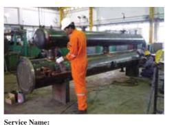
Flooded Chiller Unit Size: NPS 24" Sch 20 x 5,386mm LG x 484 tubes of 2.11mm thk MOC: SA106-GrB End user: Technical Asia
