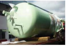
Service Name: Sulfuric Acid Tank Size: 2,000mm ID X 3,450mm T/T X 6.35mm Thk MOC: SA516-70N End user: Hyflux Malaysia
