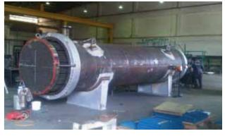
**Equipment Tag Number:** 16-E-05 Size: 1,350mm ID x 6,096mm LG x 1,818 tubes of 2.11mm Thk MOC: SA516-70N End user: Kaduna Refinery Petrochemical Co
